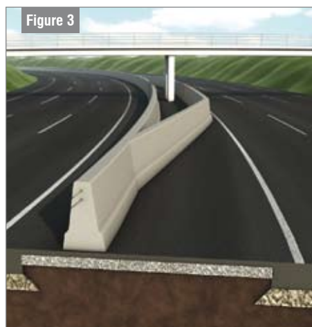
Asymmetric bifurcation at bridge pier
